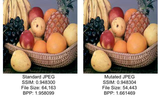
Fig. 6: Side by side comparison of a compressed sample image (from our test image set). The image was compressed with a quality factor of 80. Our method shows an improvement of more than %15 in compression ratio without degrading quality.
